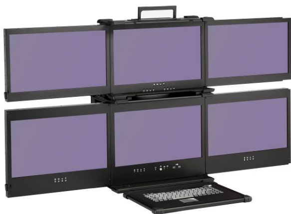
An ADP173 integrates into ARP673 to transform to 6-screens
